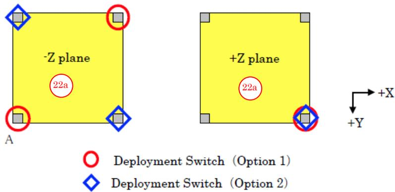
Figure 3.2.1-1 Position of Deployment Switches
