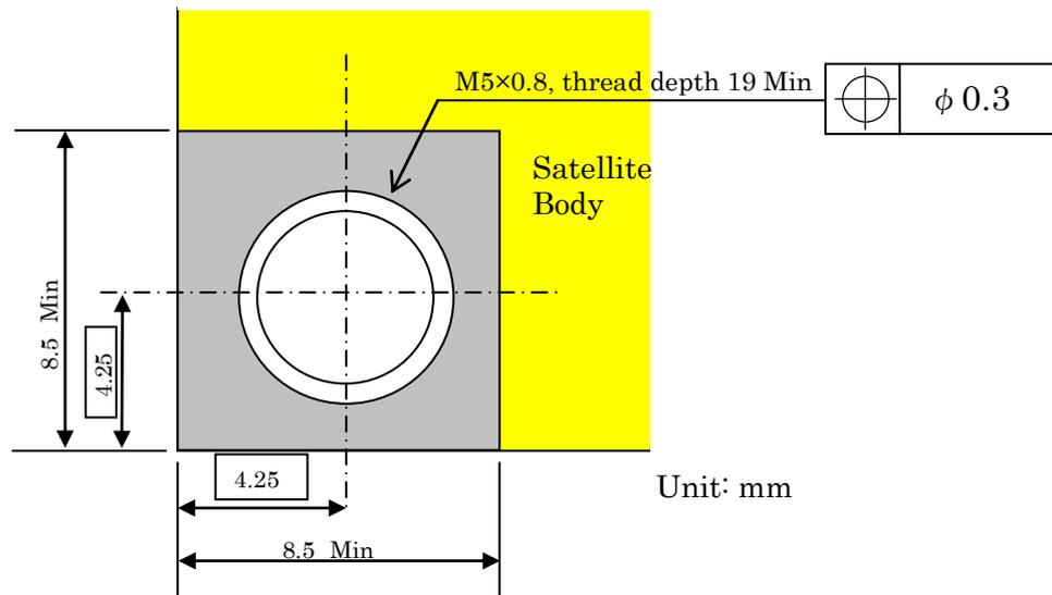
Detail A (Detail Information for Separation Spring Interface)
