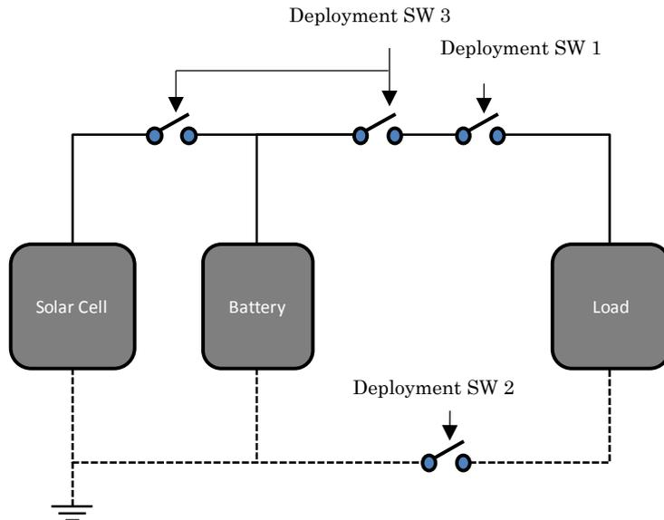
Figure 3.2.1-3 Example of three Deployment Switches
