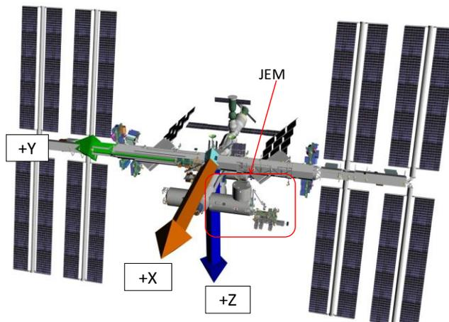
Figure A1.5-2 ISS Body Coordinate System
