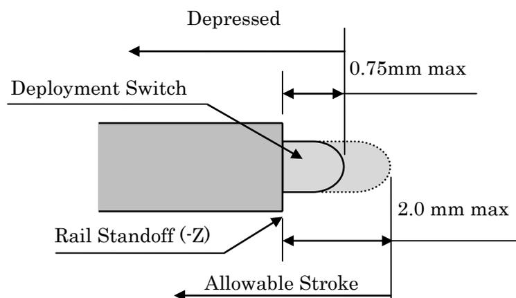
Figure 2.2.1-1 Depressed Condition and Allowable Stroke of Deployment Switches
