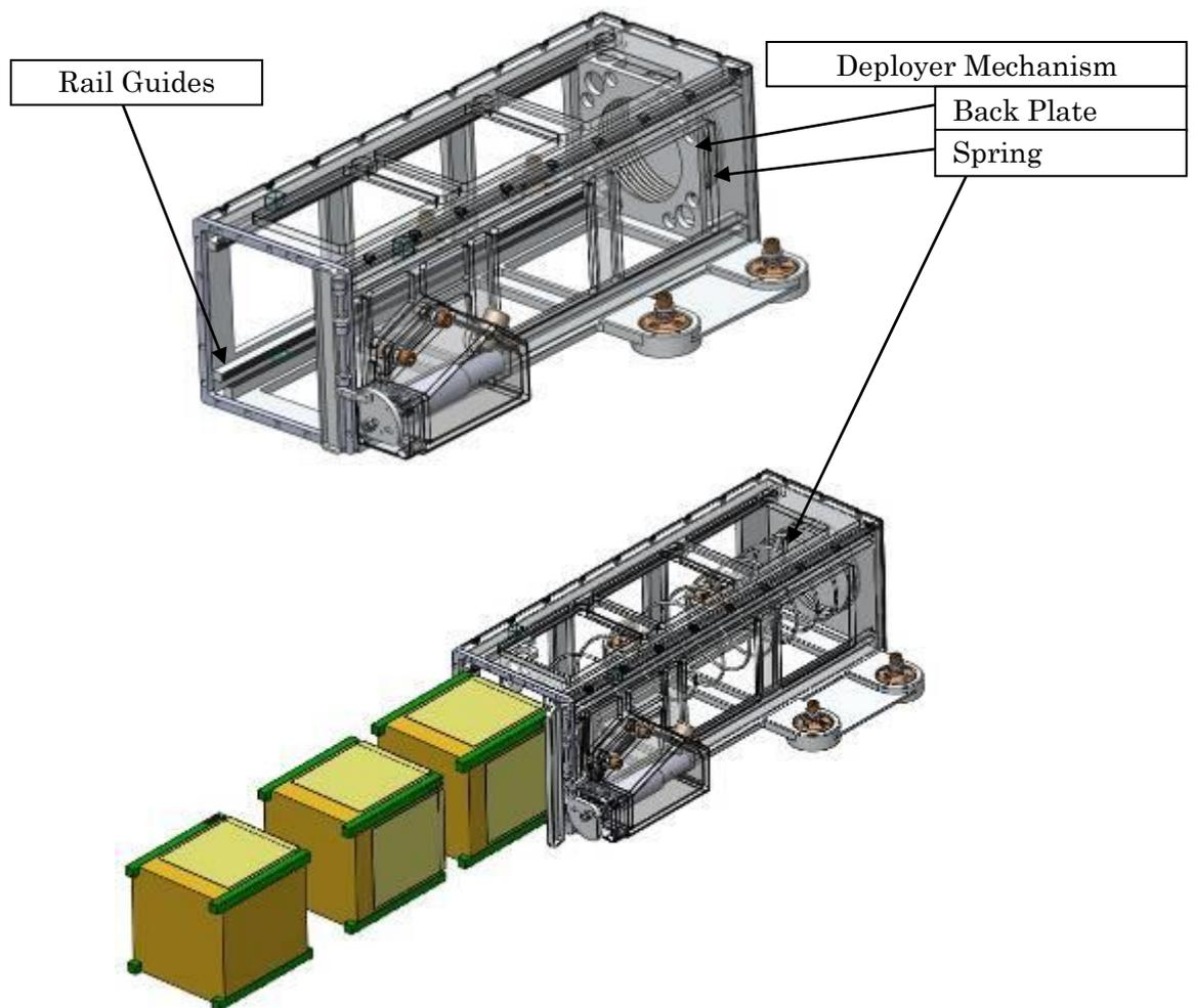
Figure A1.2-1 Satellite Install Case
