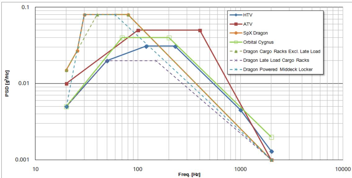
Figure 2.4.1-1 Random Vibration of each launch vehicle
