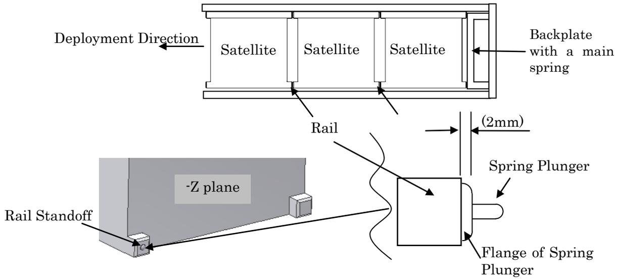
Figure 2.1.6-1 Overview of multiple satellites installation with spring plungers
