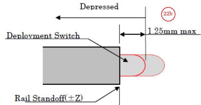
Figure 3.2.1-2 Depressed Condition of Deployment Switches
