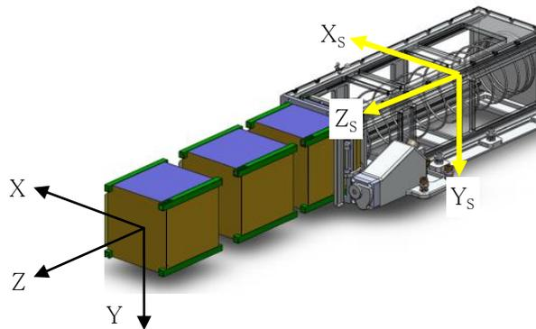
Figure 2.1.1-1 Coordinate System Definition
