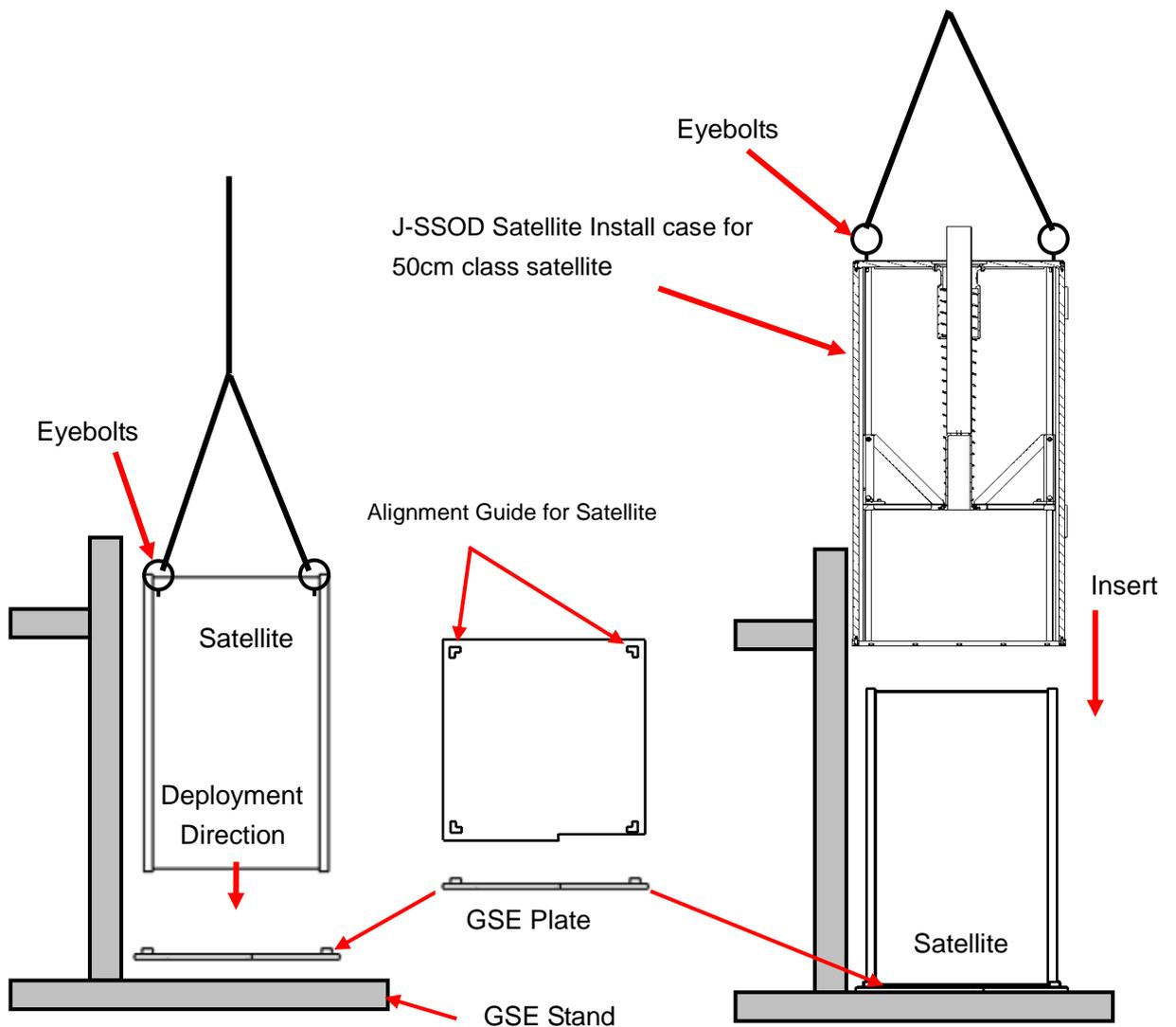
Figure 3.1.10-1 Satellite Installation into J-SSOD Satellite Install Case
