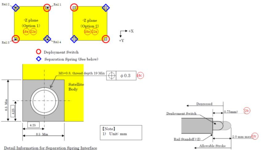
Figure 2.1.6-2 Location of Separation Spring and Deployment Switch
