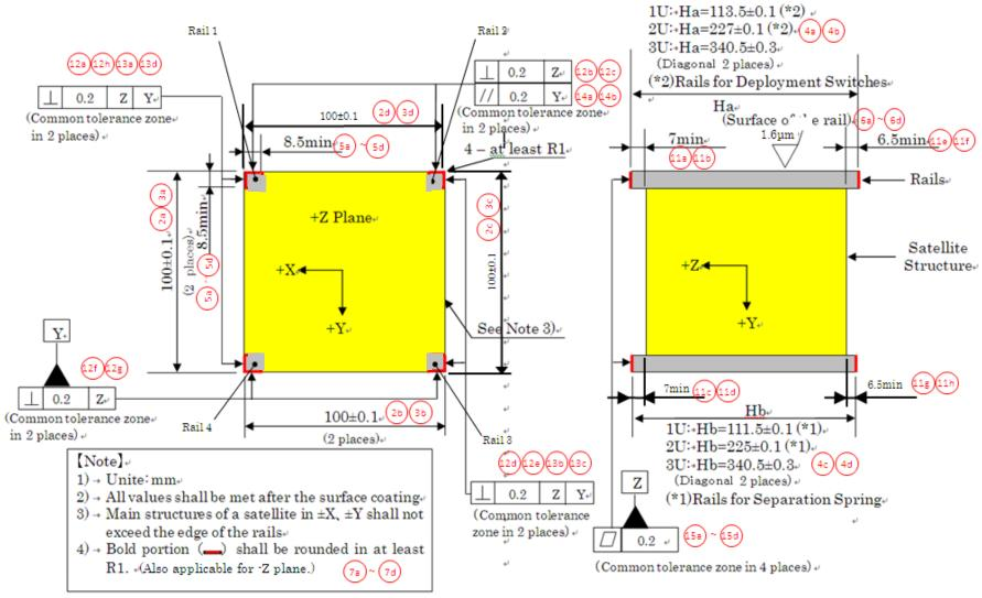
Figure 2.1.2-1 Dimensional Requierments for Satellite
