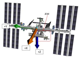
Figure A1.5-2 ISS Body Coordinate System
