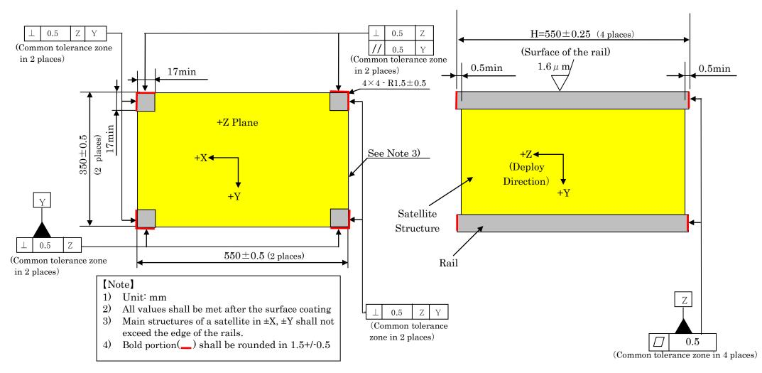
Figure 3.1.2-1 Dimensional Requirements for 50cm Class Satellite
