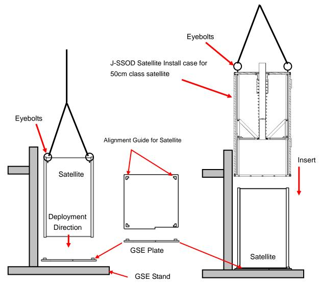
Figure 3.1.10-1 Satellite Installation into J-SSOD Satellite Install Case
