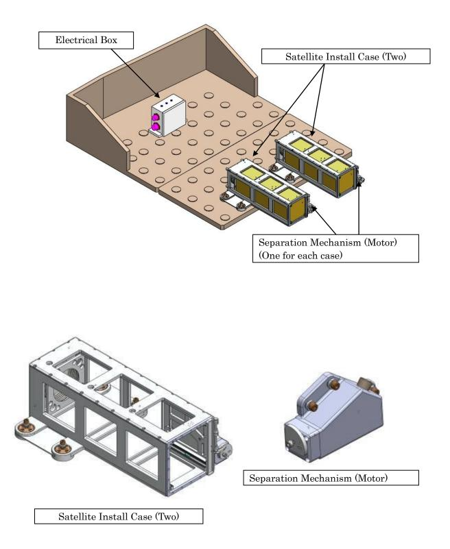
Figure A1.1-2 Major Components of Small Satellite Orbital Deployer
