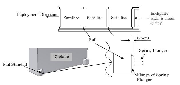
Figure 2.1.6-1 Overview of multiple satellites installation with spring plungers
