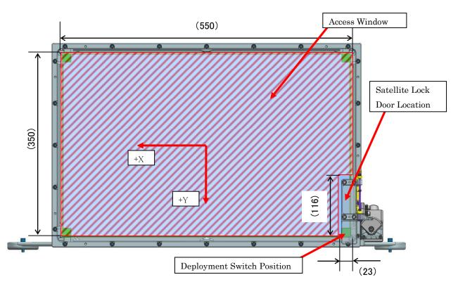
Figure 3.1.7-1 Satellite Access Window after removal of Launch Lock Cover
