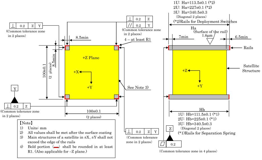
Figure 2.1.2-1 Dimensional Requierments for Satellite
