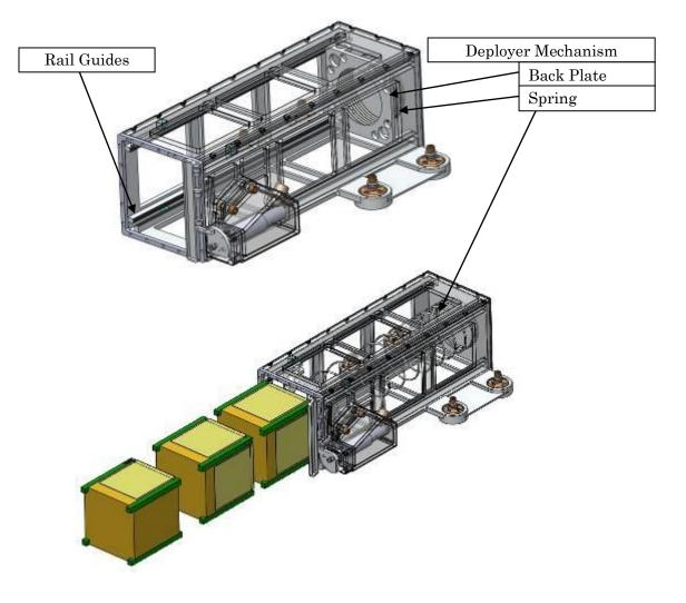
Figure A1.2-1 Satellite Install Case
