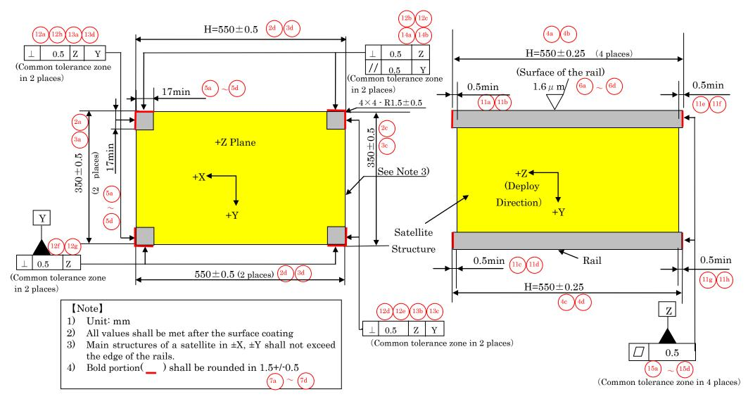
Figure 3.1.2-1 Dimensional Requirements for 50cm Class Satellite
