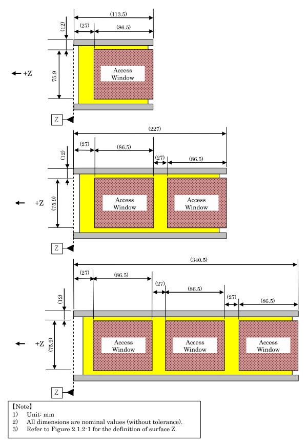
Figure 2.1.7-1 Nominal Position of Access Window in -Ys(-Y)/+Xs(+X)
