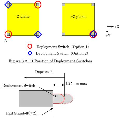
Figure 3.2.1-2 Depressed Condition of Deployment Switches
