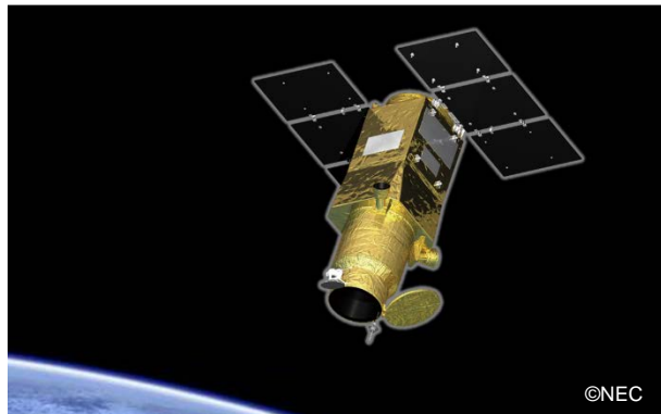
ASNARO-1 Small-sized High-resolution Optical Satellite using NX-300L
