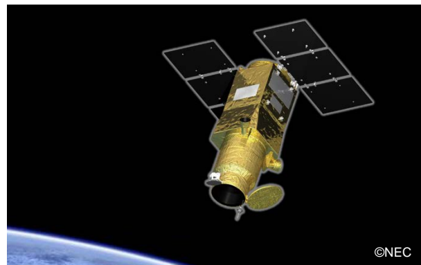
ASNARO-1 Small-sized High-resolution Optical Satellite using NX-300L
