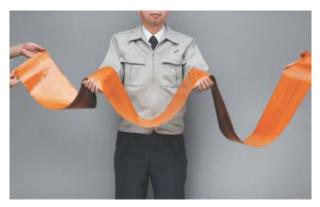
Long FPC Extended up to 100 meters. Used in JAXA's solar power sail demonstration aircraft "IKAROS".
