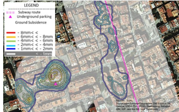
Surface Motion Monitoring service for underground construction Monitoring subsidence along construction period by using SAR satellite imagery.
