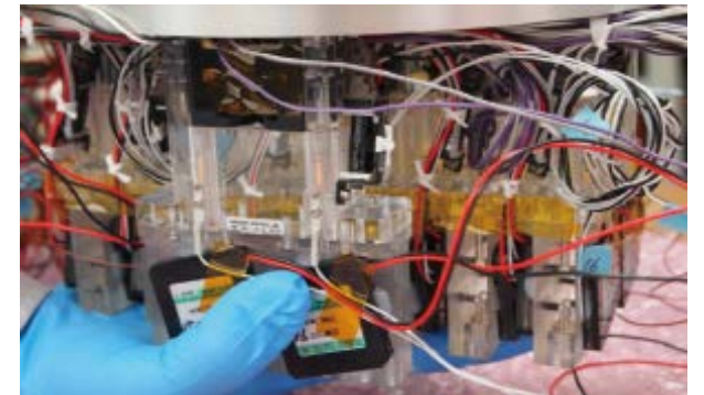
Ultra Small valves and Pumps Adopted in a liquid mixing system for a microgravity experimental device in a JAXA observation rocket in 2012.
