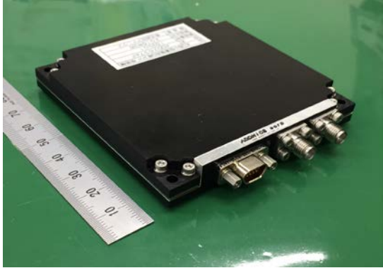
A88 S-band Receiver 2050-2100MHz, PCM-PSK-PM, 4kbps 80 X 80 X 16mm / 130g
