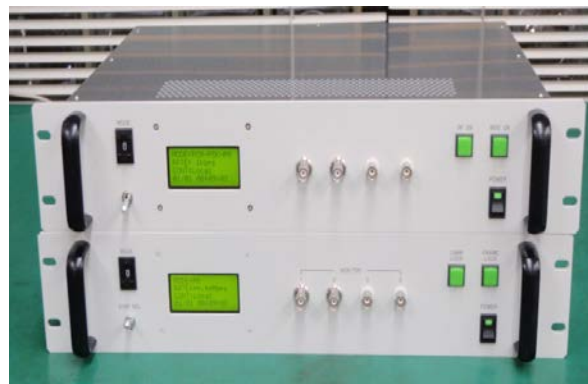
S/X-band Ground Station Command Signal Generator Telemetry Receiver – Demodulator Data Receiver – Demodulator
