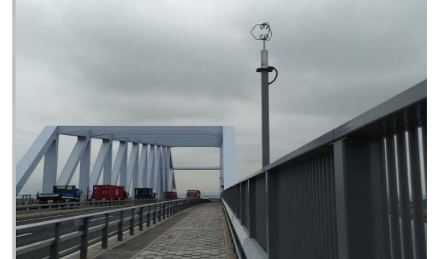
3D ultrasonic anemometer Wind monitoring including up-wash and downwash at bridge etc.
