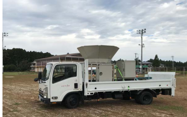
Portable Doppler SODAR 3-D wind profile monitoring for wind resource assessment of wind power generation and UAV operation control
