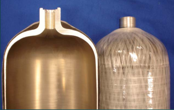
Liners for High Pressure COPVs From R&D to High Production
