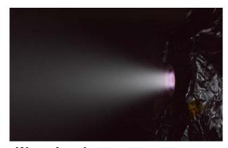
Water ion thruster 152 – 460 μN, 560 – 1452 s, 22 – 62 W, 1.6 kg (dry), 0.7U (w/o tank)
