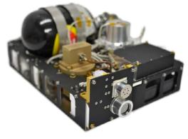
Satellite: HODOYSHI-4 (60 kg-class) Launcher: Dnepr in 2014 Propulsion type: Ion (Flight Proven)
