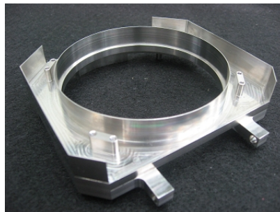
Super invar cutting workpiece a low thermal expansion alloy also used for observation equipment; super invar alloy shaving
