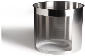
Thin stainless steel ring(SUS304) Lightweight products using thin-walled. Precision composite cutting technology. It is a thin ring of \phi 380 \times 350 L \times t1 . (Circularity 0.1).
